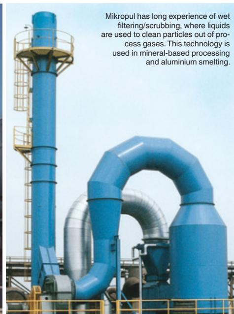
Mikropul has long experience of wet filtering/scrubbing, where liquids are used to clean particles out of process gases. This technology is used in mineral-based processing and aluminium smelting.
